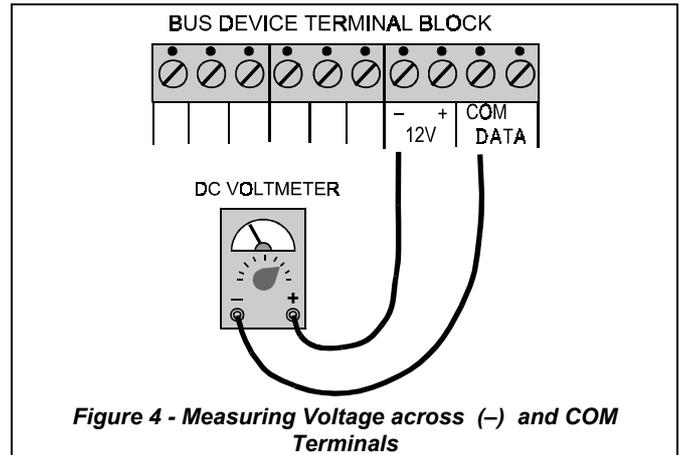
Figure 4 - Measuring Voltage across (-) and COM Terminals
