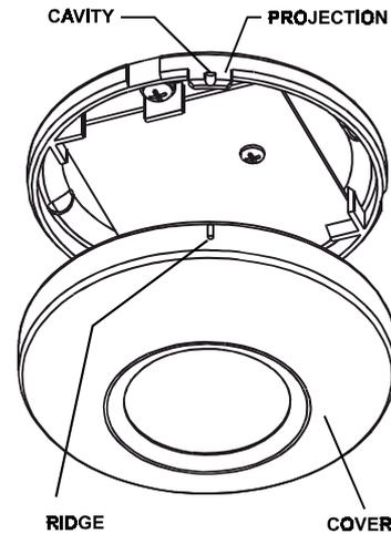
Figure 4-6. Installing the Cover
