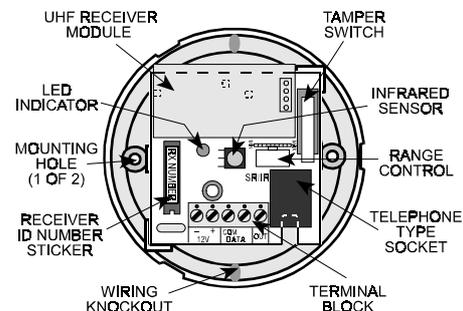
Figure 4-2. Receiver with Cover Removed
