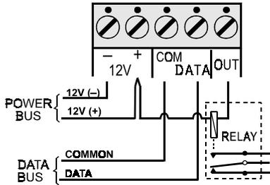
Figure 4-3. Terminal Block Connections
